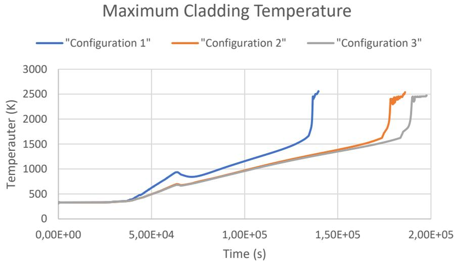
**Figure 6, Evolution of Maximum Cladding Temperatures in Different Configurations**
