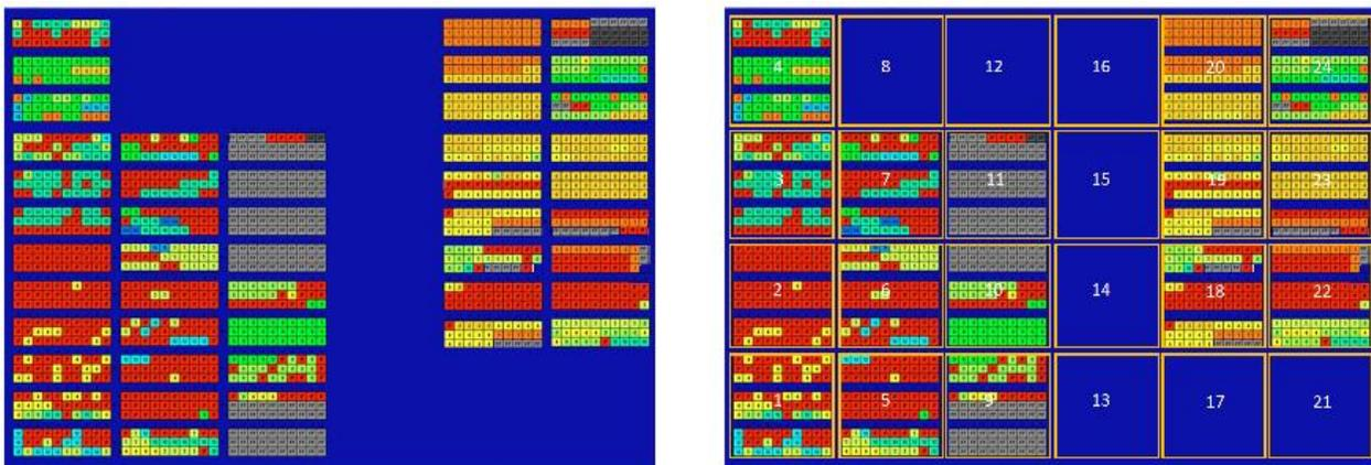
**Figure 2, Spent Fuel Pool Nodalization Using the Flexible Nodalization Method**
