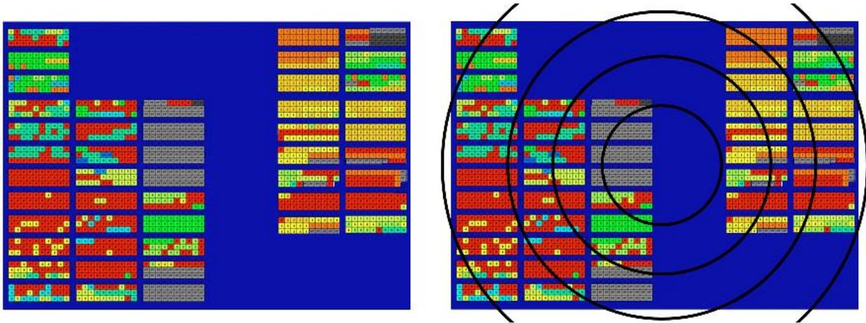
**Figure 1, Spent Fuel Pool Nodalization Using the Standard Ring-Like Method**
