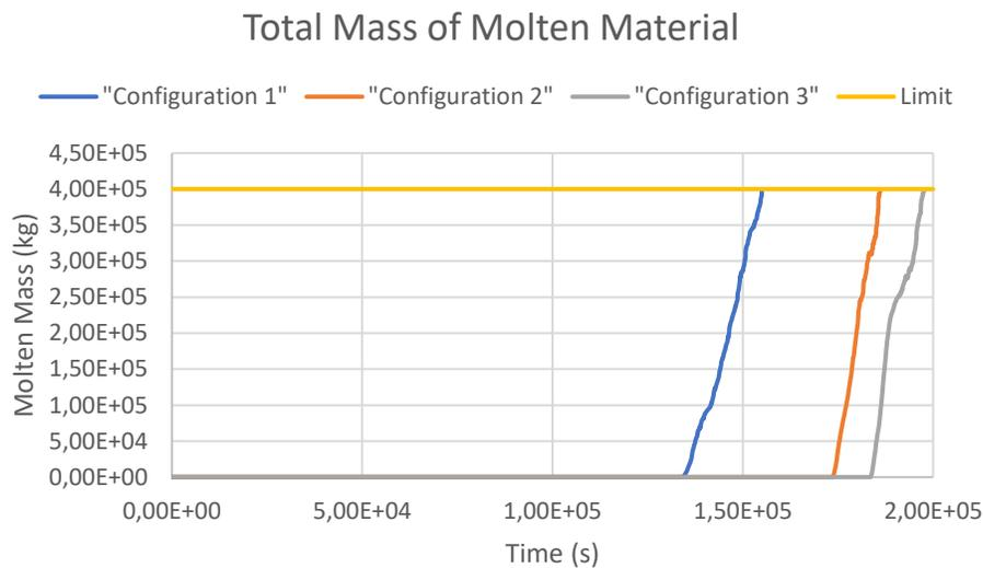
**Figure 7, Evolution of Molten Mass in Different Configurations**
