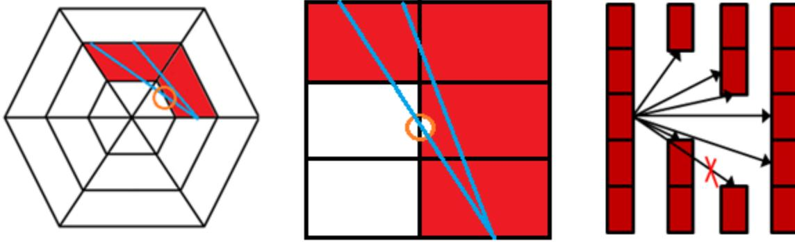
**Figure 3, Top and Side View of a Partially Molten Reactor / Spent Fuel Pool Using the Flexible Nodalization - Heat Radiation Paths with Shadowing -**
