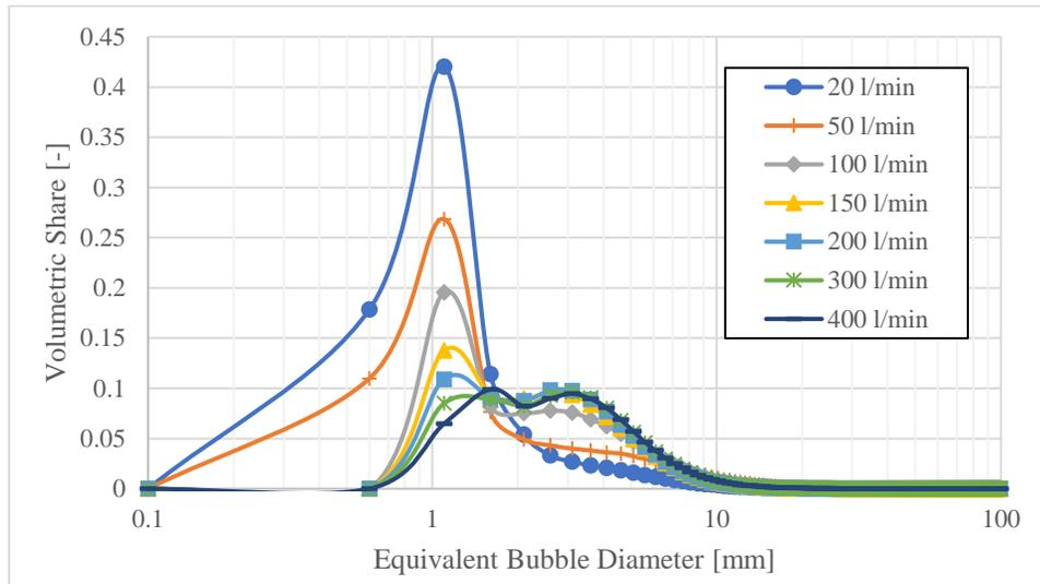
Figure 5. Volumetric share of the bubbles in dependence of the equivalent bubble diameter at a distance of 842 mm from the CCI injector with the mixing element for different flow rates at adiabatic temperature conditions.
