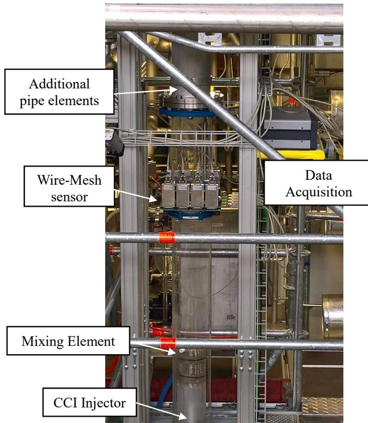
Figure 4. ISOLDE test facility with WMS data acquisition system, the CCI injector with mixing element and the additional pipe compartments on the top.
