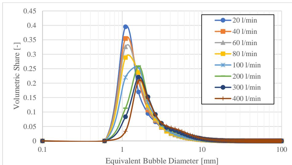
Figure 6. Volumetric share of the bubbles in dependence of the equivalent bubble diameter at a distance of 722 mm from the CCI nozzle without the mixing element for different flow rates at adiabatic temperature conditions.
