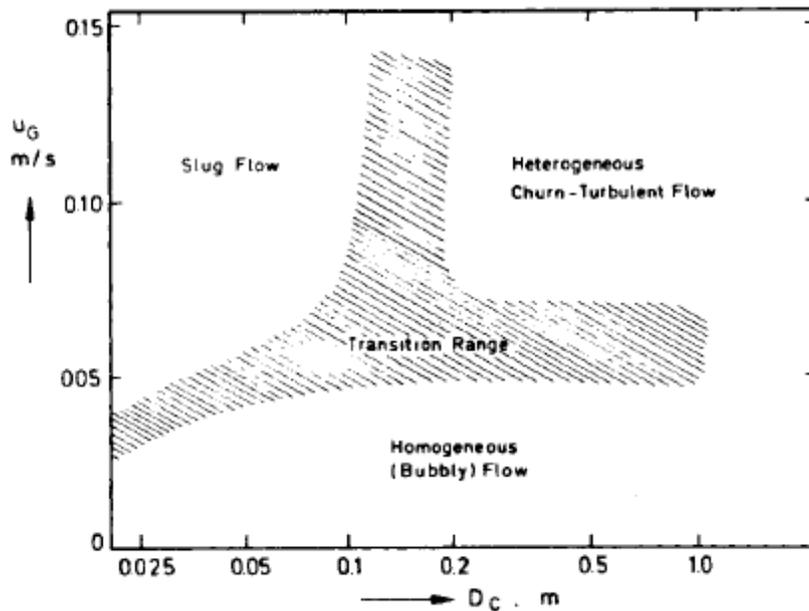
Figure 7. Approximate dependence of flow regime on gas velocity and column diameter (water and dilute aqueous solutions) [15].
