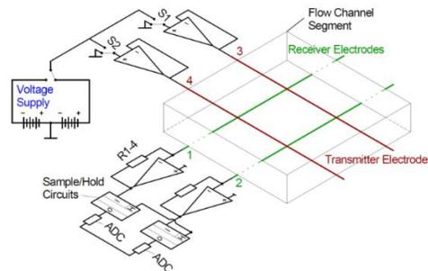
Figure 3. Electrical schematic of the wire-mesh sensor [10].
