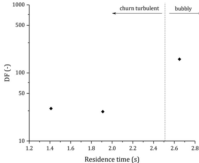
Figure 2. DF as a function of residence time showing significant change in the flow regime transition using the injector and mixing element from CCI-IMI-Nuclear and loaded with 0.06 M  $\text{Na}_2\text{S}_2\text{O}_3$  and 0.1 M NaOH at 21 °C in the mini-VEFITA test facility [7].
