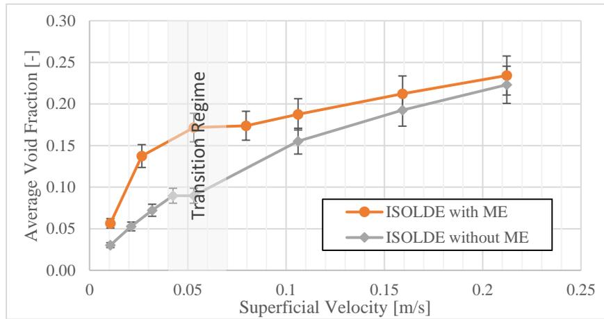
Figure 8. Evolution of average void fraction for different gas flow rates compared and the distinction between bubbly and churn-turbulent flow at adiabatic temperature.
