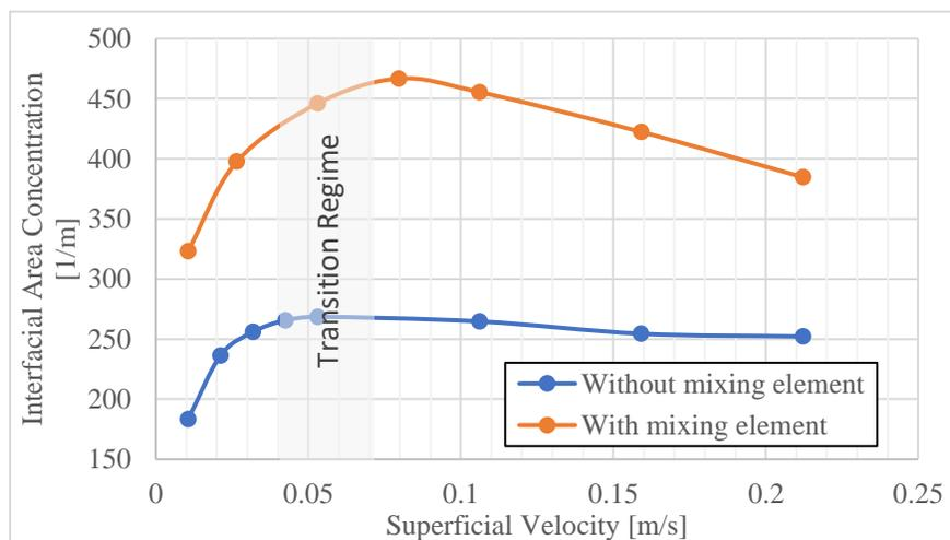
Figure 9. Interfacial area concentration for different flow rates with the CCI injector with and without mixing element at adiabatic temperature conditions.
