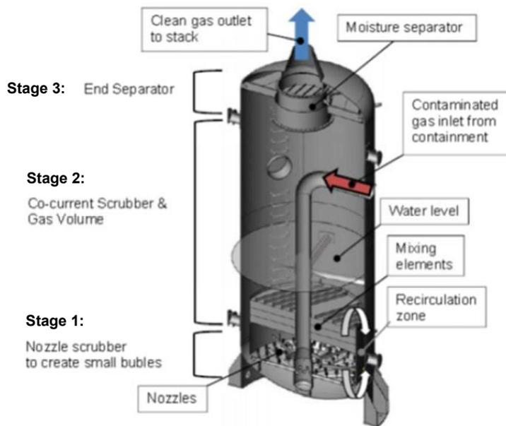
Figure 1. Schematic of the CCI-IMI-Nuclear Scrubber [1].
