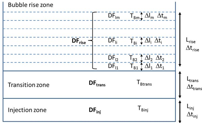
**Figure 1** Zones and meshes of the water pool considered for DF evaluation
