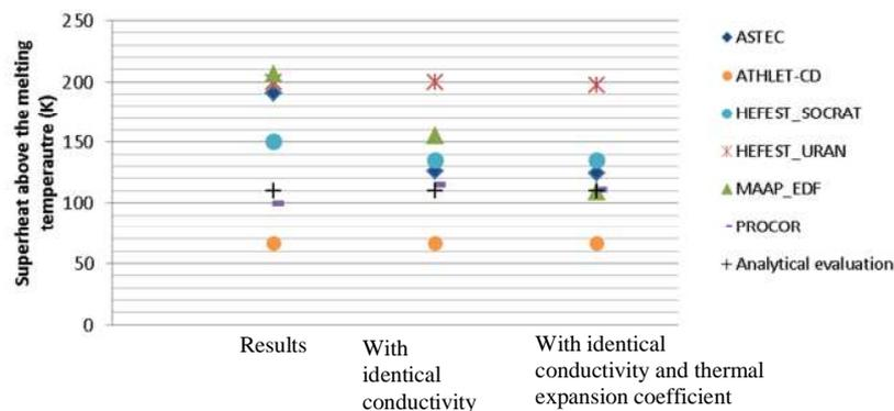
Figure 5 Oxide superheat and impact of dispersion in material properties (analytical evaluation being considered here as reference)
