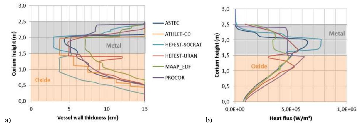
Figure 10 Profiles of ablated vessel wall (a) and heat flux (b) at steady state<sup>8</sup> (case n°3)
