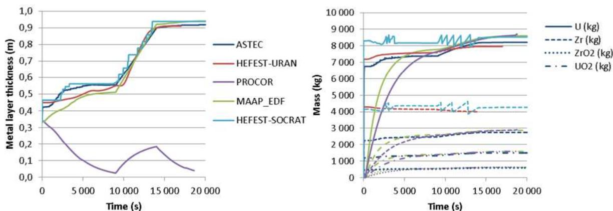
Figure 13 Evolution of the thickness (left) and of the composition<sup>10</sup> (right) of the top metal layer (case n°4)
