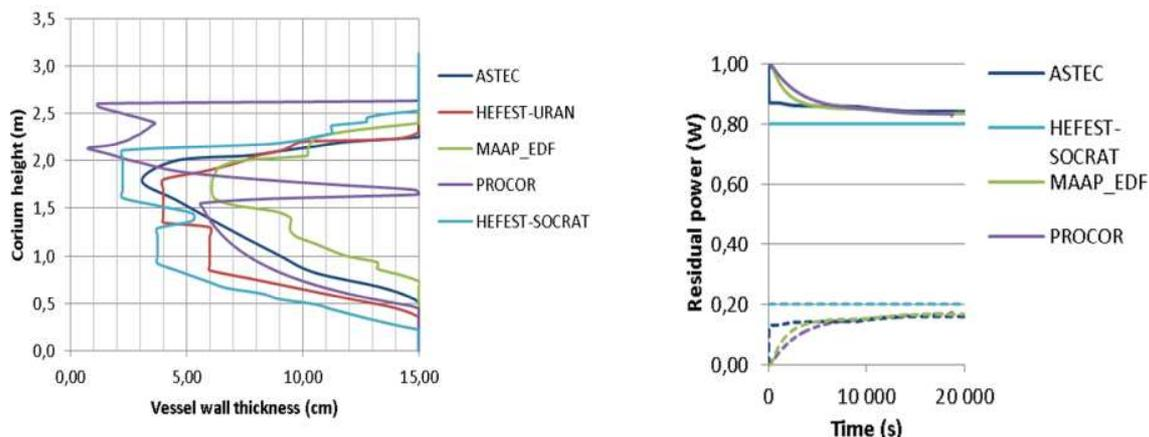
Figure 12 Ablated vessel wall at steady state (left) and residual power distribution between oxide (full lines) and metal (dashed lines) phases<sup>9</sup> (right) (case n°4)
