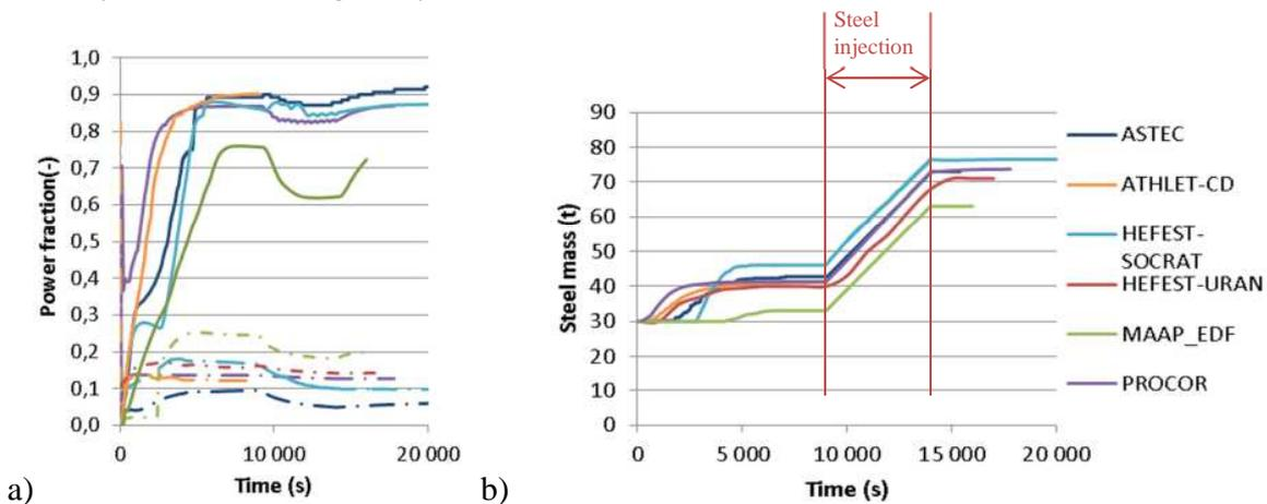
**Figure 9 a) Fraction of residual power dissipated by the external cooling<sup>7</sup> (full lines) and by the radiation at the top of the pool (dashed lines); b) Evolution of the mass of molten steel incorporated in the metallic layer (case n°3)**
