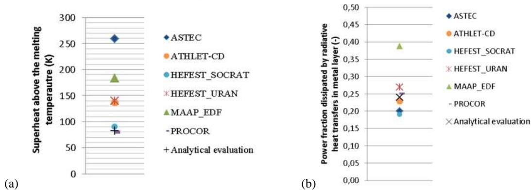
Figure 7 Metal superheat (a) and power fraction dissipated by radiation in the metal (b) in case n°2
