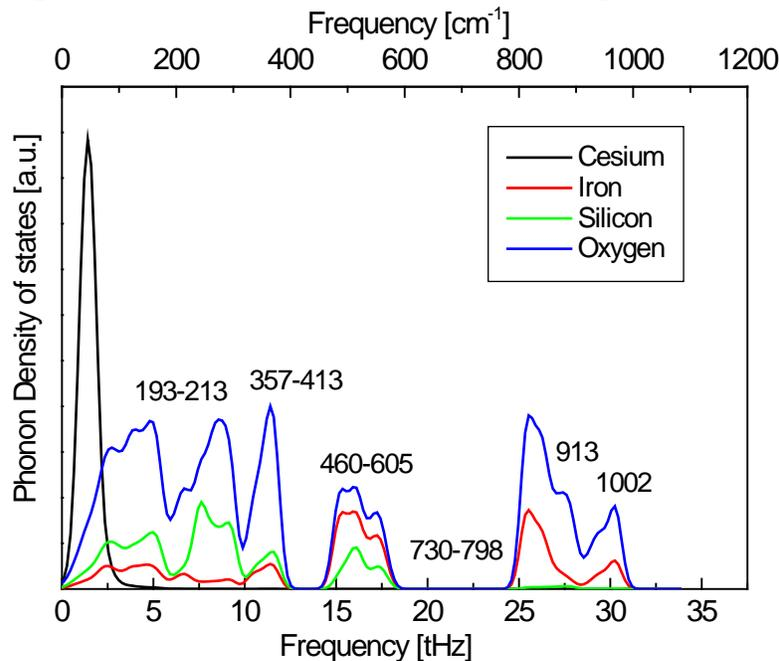
**Figure 7. Phonon Density of states calculated for  $\text{CsFeSiO}_4$ .**
