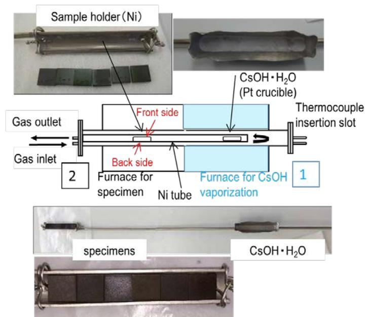
Figure 1. Illustration of CREST apparatus [14].
