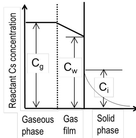
**Figure 4. Illustration of the penetration image around the gas-solid interface.  $C_g$  is the initial CsOH concentration,  $C_w$  the concentration of Cs reactive species at the interface between the gas phase and solid phase (gas film),  $C_i$  the concentration of Cs reactant species in the solid phase at the interface [17].**
