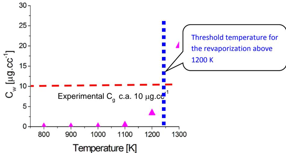
**Figure 8. Estimated partial pressure near the gas-solid interface ( $C_w$ ) in the case of  $p(\text{H}_2)=0.05\text{bar}$  and  $(\text{H}_2\text{O})=0.0005\text{bar}$ .**
