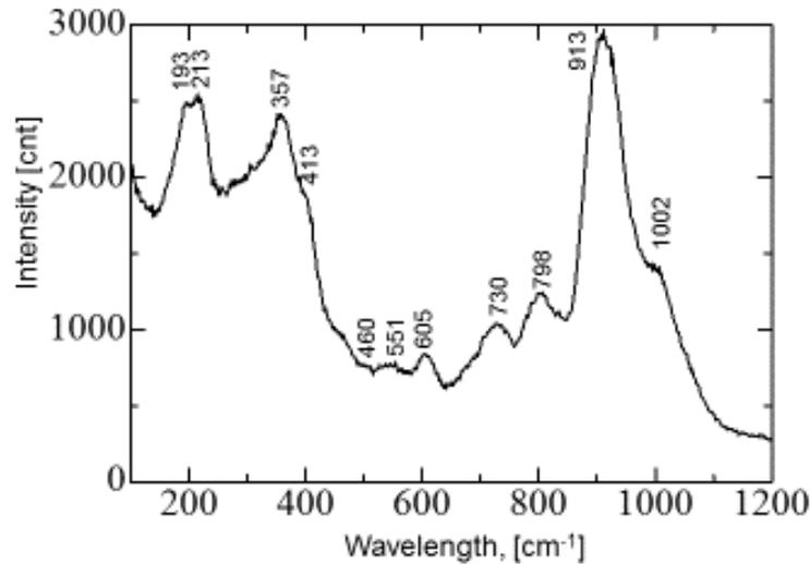
**Figure 6. Raman shift of  $\text{CsFeSiO}_4$  at room temperature [15].**
