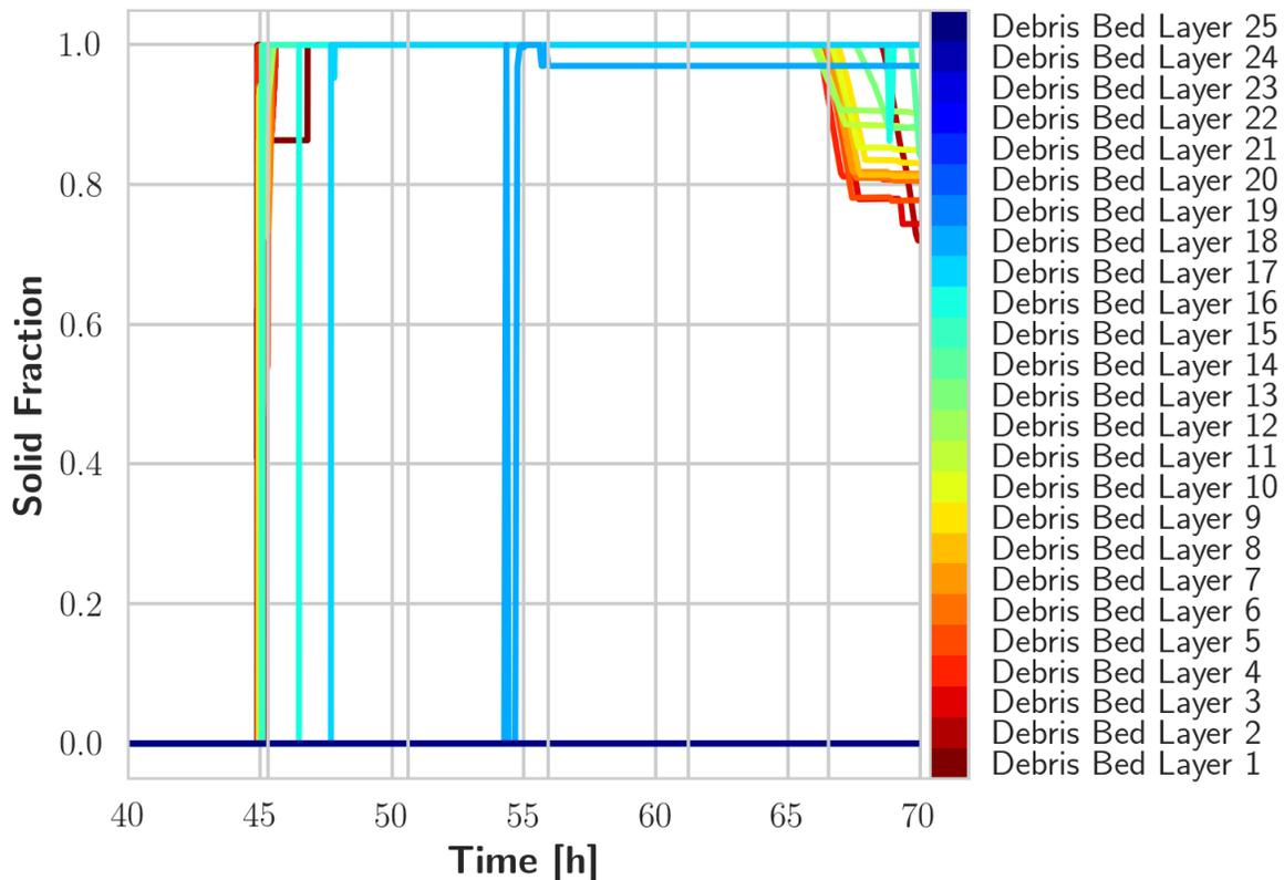
Figure 5 - 1F3 Like Lower Plenum Debris Bed Axial Solid Fraction
