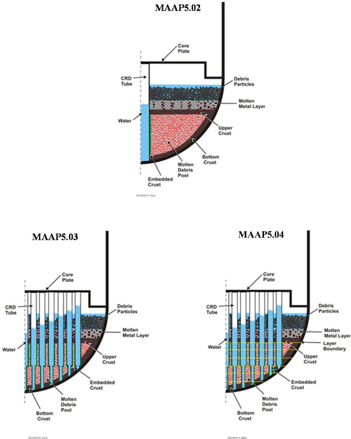
Figure 1 - Lower Plenum Model Evolution
