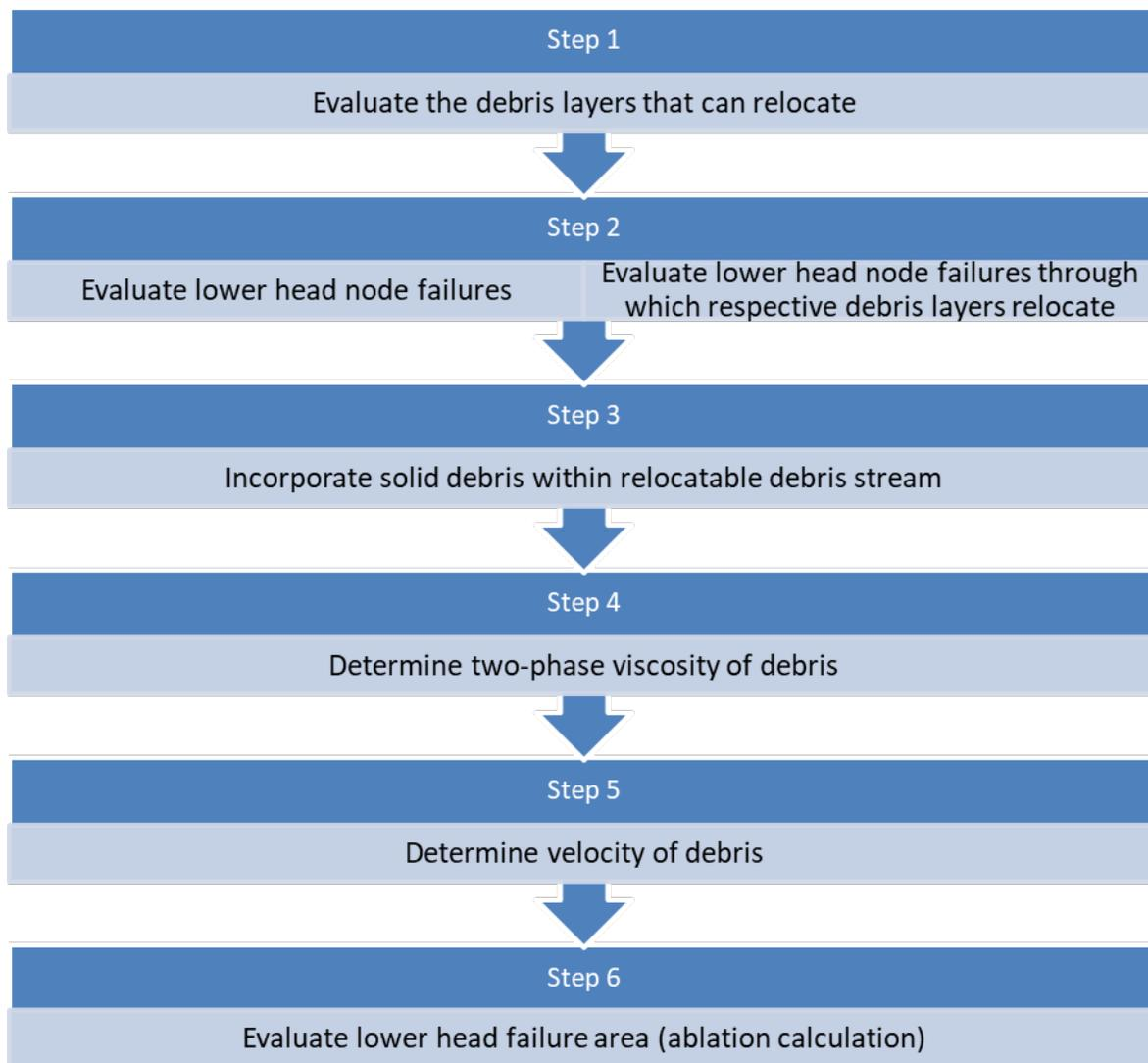
Figure 6 - Evaluation Steps for Ex-Vessel Debris Relocation Module
