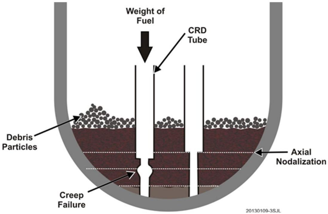
Figure 4 - CRD Tube Creep
