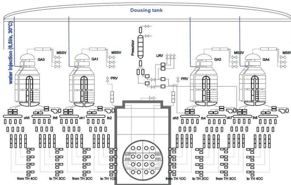
Figure 7. SGs depressurization and water injection model
