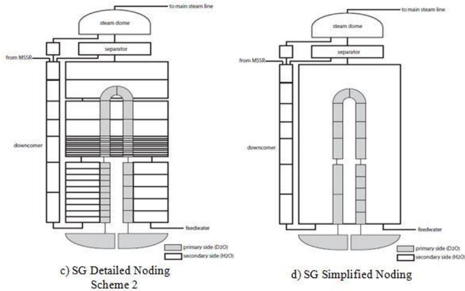
**Figure 4. Proposed nodalization for the SGs in a SBO analysis**
