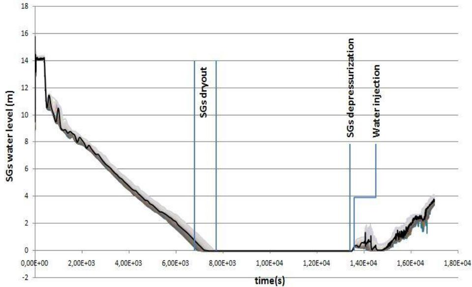
Figure 15. Water level in the secondary side of the SGs
