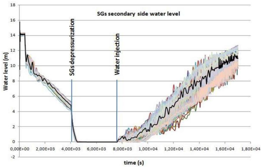
Figure 12. Water level in the secondary side of the SGs
