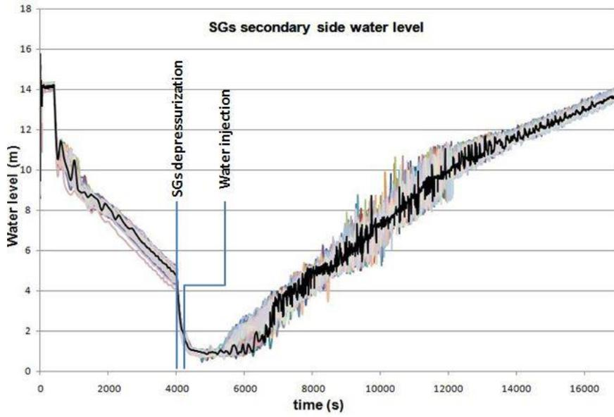
Figure 9. Water level in the secondary side of the SGs
