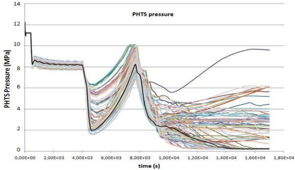
Figure 11. Pressure of the coolant in the primary system
