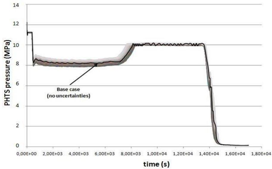
Figure 14. Pressure of the coolant in the primary system
