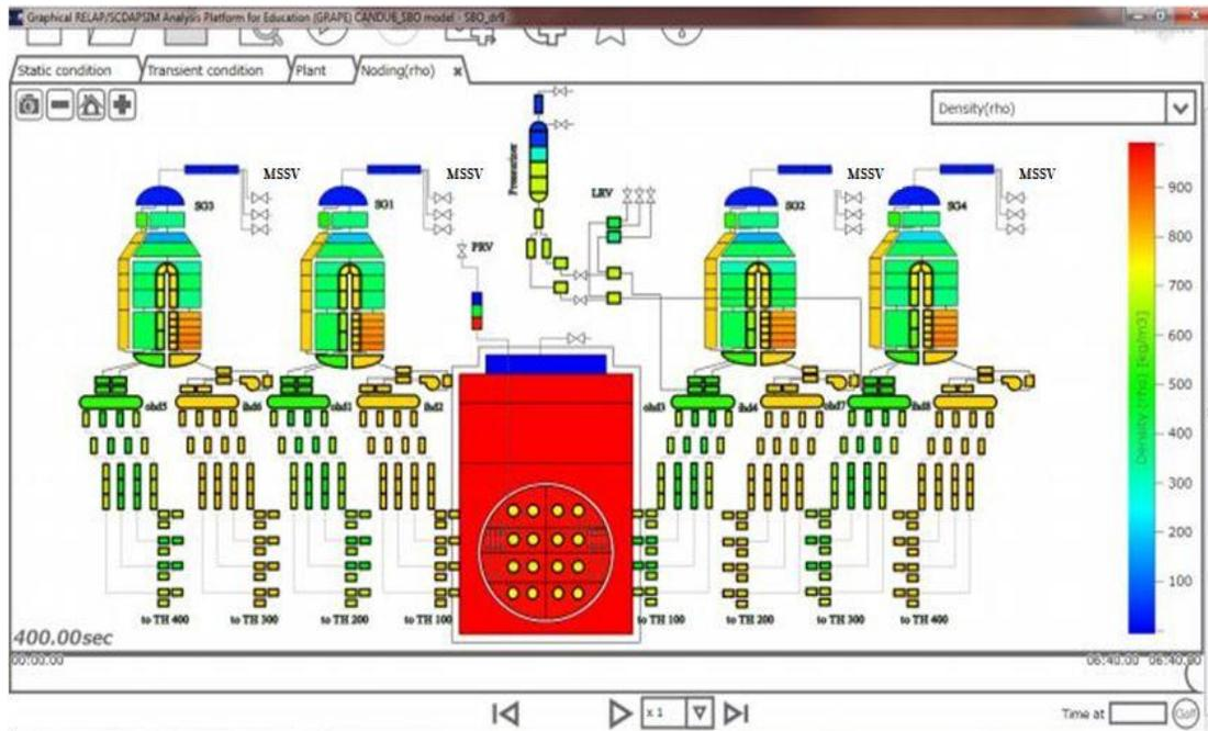
Figure 3. CANDU 6 model for the SBO accident analysis<sup>1</sup> [18]
