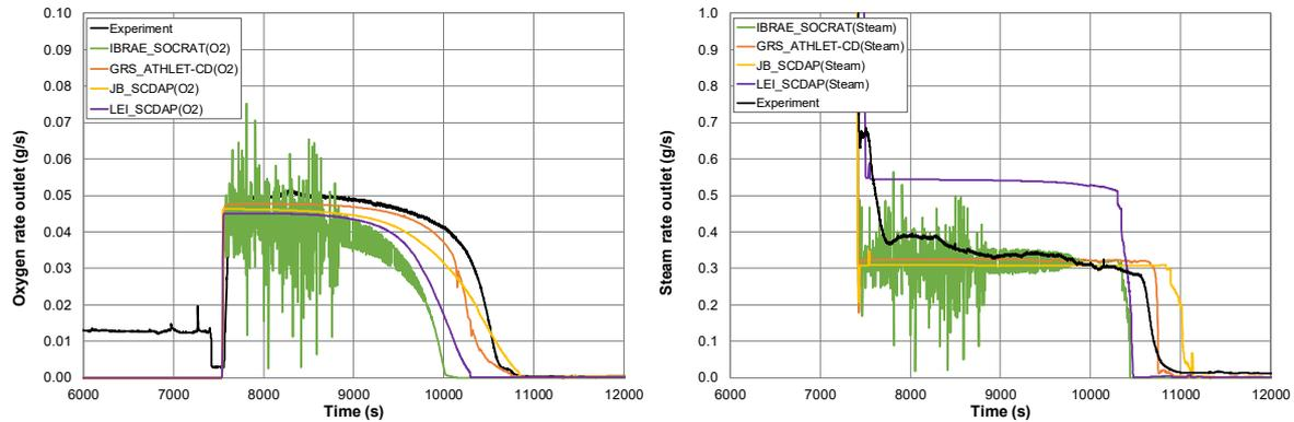
Figure 8, Measured and calculated oxygen (left) and steam flow rate (right) at the outlet
