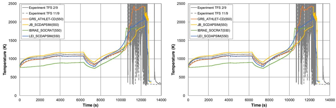
Figure 6, Measured and calculated cladding temperatures at 350 mm (left) and 550 mm (right)
