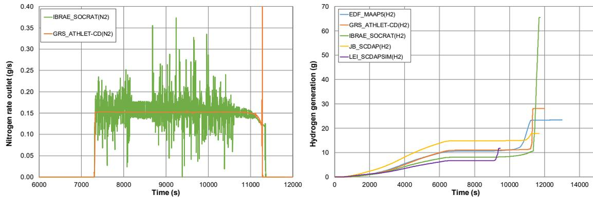
**Figure 5, Calculated nitrogen flow rate at the outlet (left) and hydrogen generation (right) of the pre-test benchmark**
