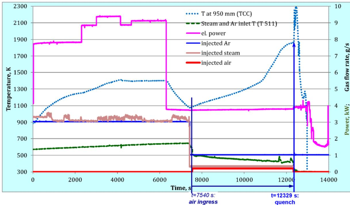
Figure 2, QUENCH-18 test conduct [2]
