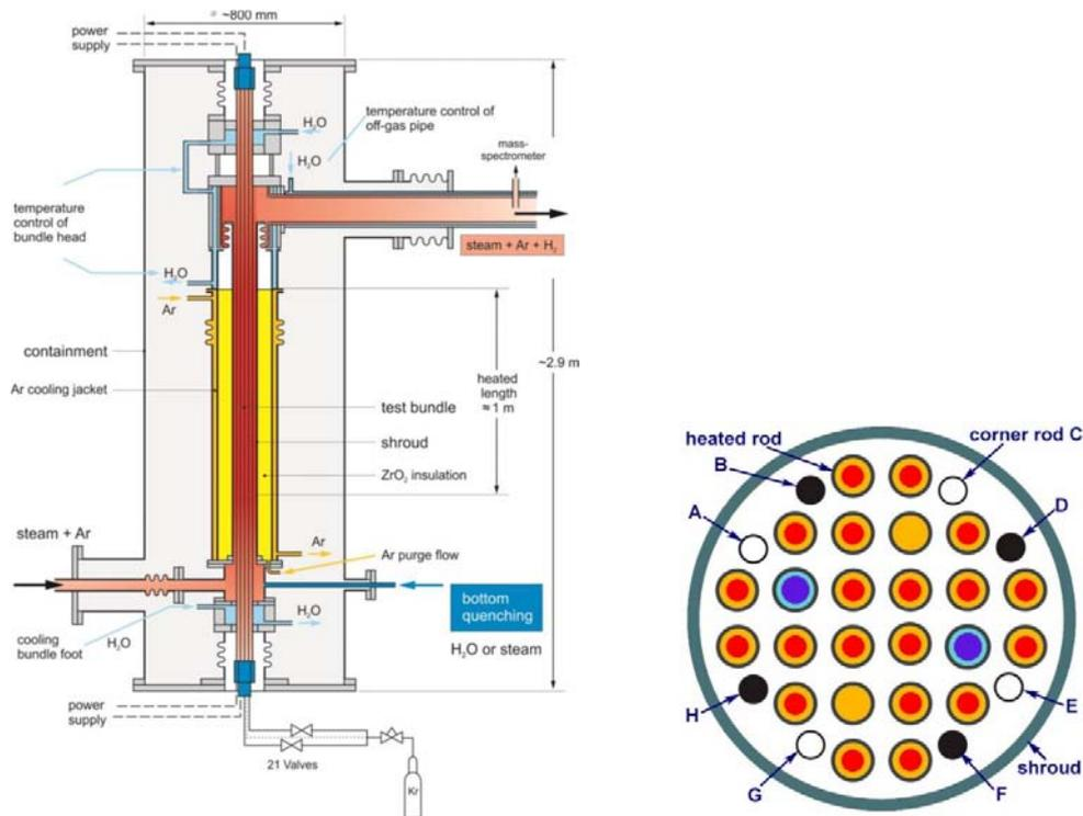
Figure 1, QUENCH facility (left) [3] and bundle (right) [2]
