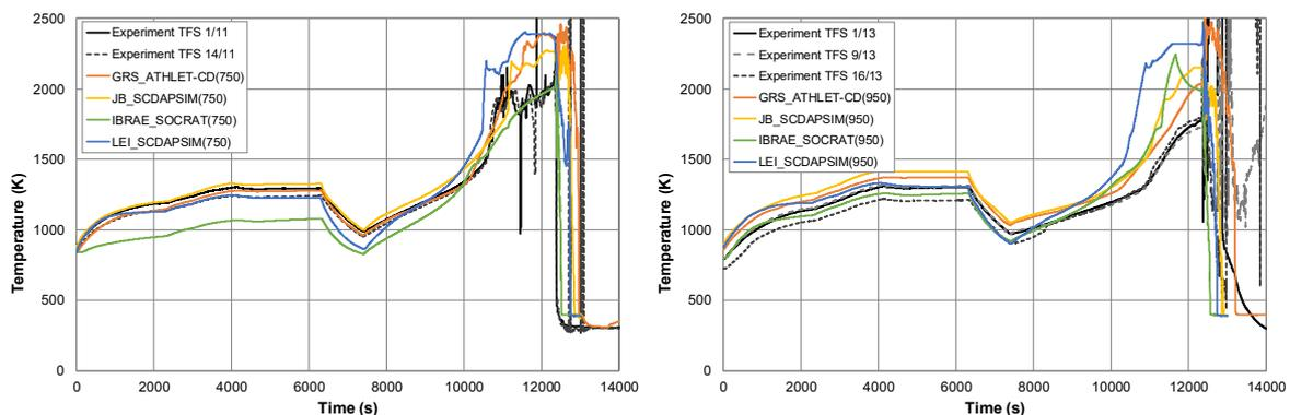
Figure 7, Measured and calculated cladding temperatures at 750 mm (left) and 950 mm (right)
