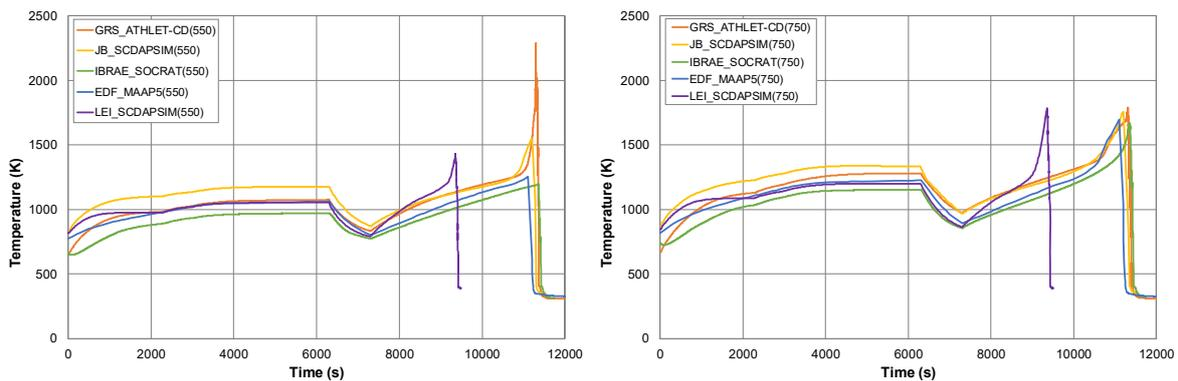
**Figure 3, Calculated cladding temperatures at 550 mm (left) and 750 mm (right) of the pre-test benchmark**
