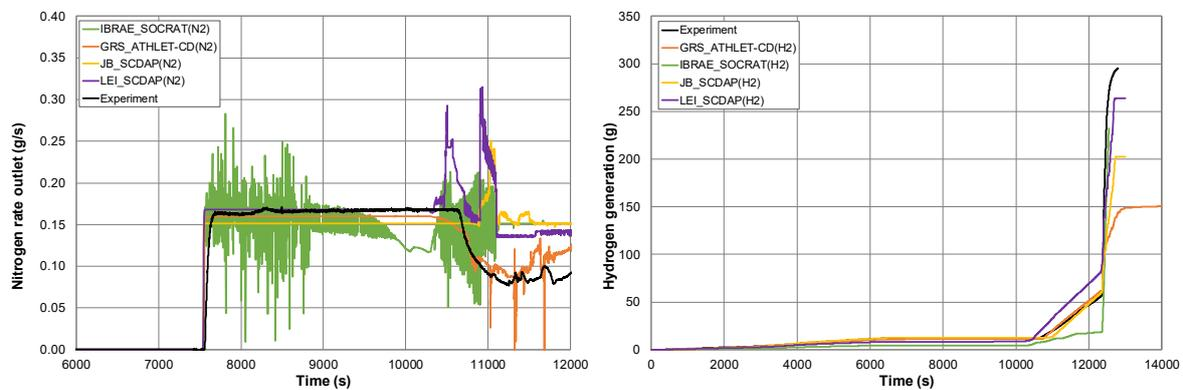
Figure 9, Measured and calculated nitrogen flow rate at the outlet (left) and hydrogen generation (right)
