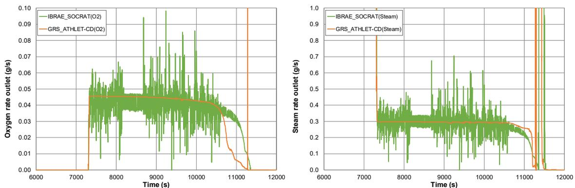
**Figure 4, Calculated oxygen (left) and steam (right) flow rate at the outlet of the pre-test benchmark**
