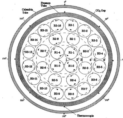
Figure. 3. Cross-sectional view of CS28-1 experimental test section.
