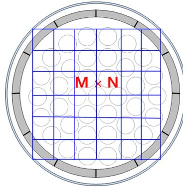
Figure. 2. Node system for a fuel channel in CAISER
