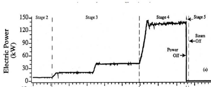
Figure. 4. Electric power to the heater in CS28-1 experiment
