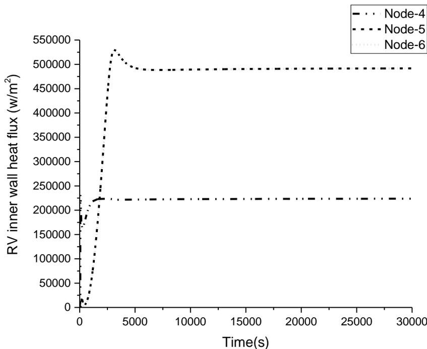
**Figure 3 Heat flux from the Corium Pool to the RV Inner Wall**
