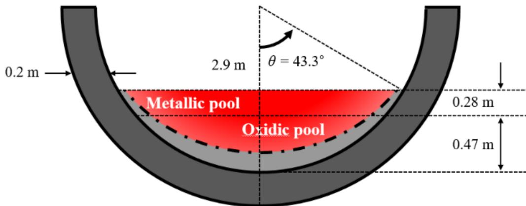
**Figure 2 Two Corium Layers Formed in Reactor Vessel Lower Plenum**
