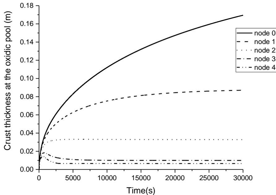
Figure 4 Crust thickness at the oxide pool
