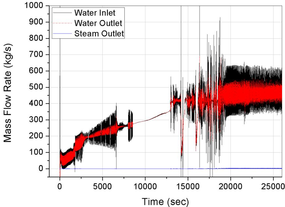
**Figure 5 SPACE Result of Coolant Circulation Flow**
