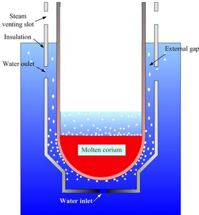
Figure 1. Conceptual design of SMART ERVC.
