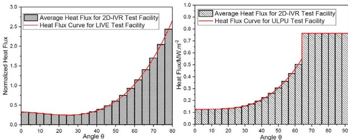
**Figure 9. Heat flux profile definition, left, LIVE-HF profile, right, ULPU profile**
