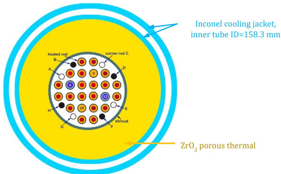
Figure 2. Cross-section of the QUENCH-ALISA bundle
