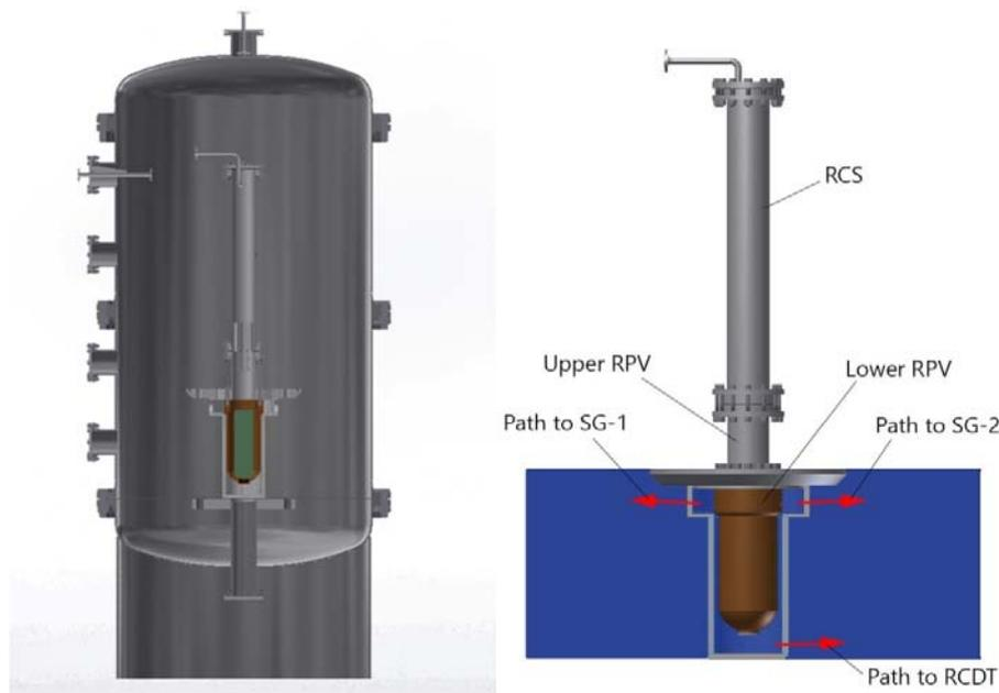
**Figure 4. DISCO facility and the test configuration in ALISA test**
