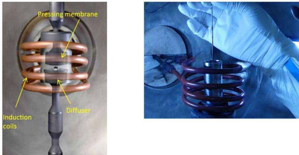
Figure 7. VITI levitation (left) and VITI-MBP setups (right)
