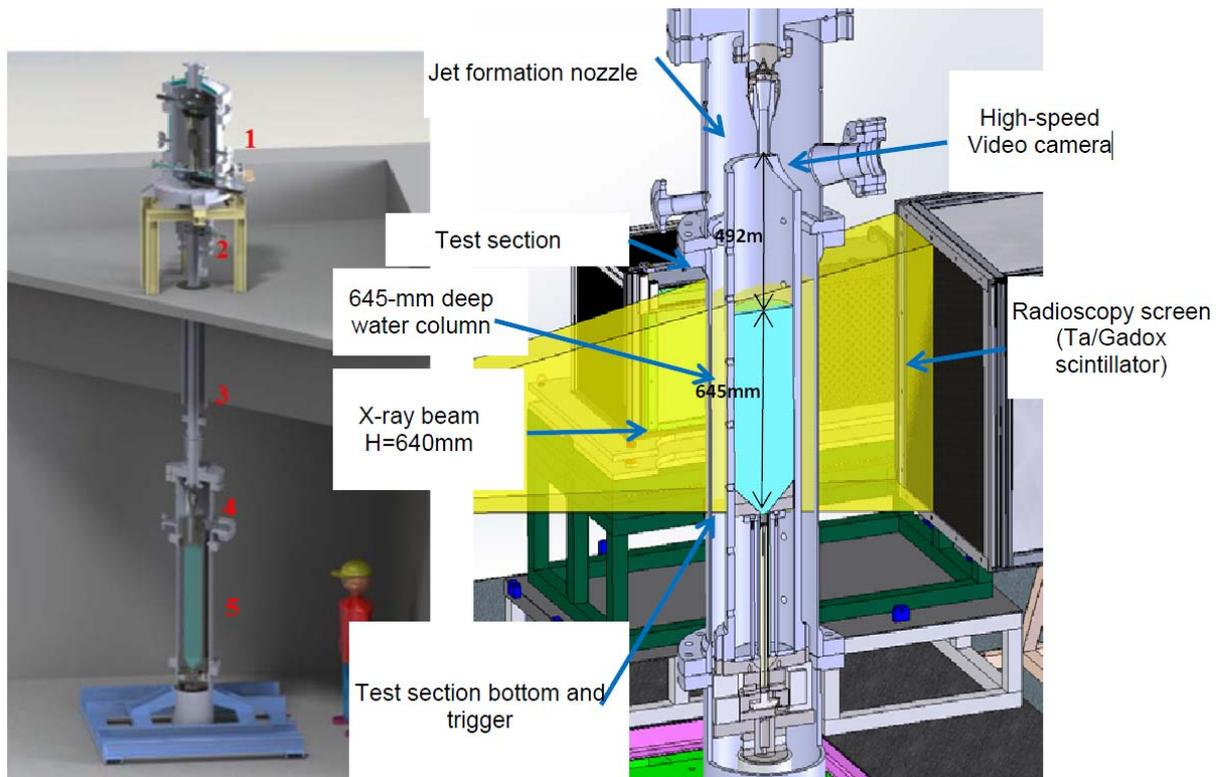
**Figure 6. KROTOS facility: Left: general sketch (deep water configuration) – Right: zoom on test section (shallow water configuration)**
