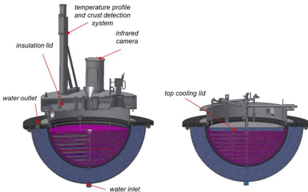
Figure 3. LIVE test facility with top insulation (left) and top cooling (right) conditions.
