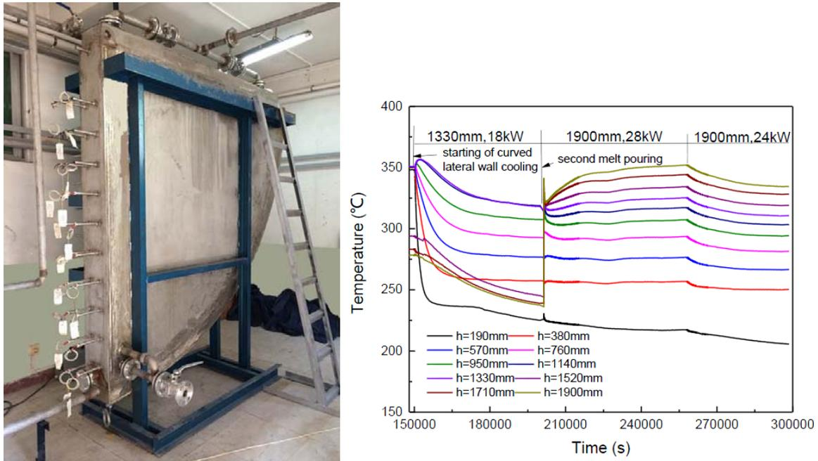
**Figure 10. Left: test vessel of the COPRA facility, right: melt temperature response during the transient phases**
