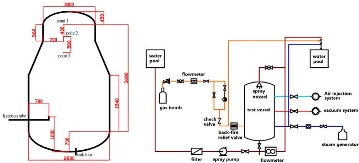
Figure 13. Sketch of MCTHBF vessel and the auxiliary components
