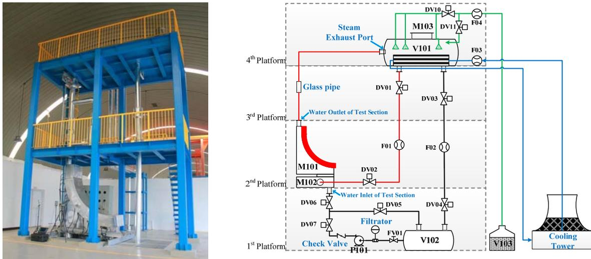
**Figure 8. Left: IVR-2D facility and test section, right: Schematic diagram of primary system of test facility.**
