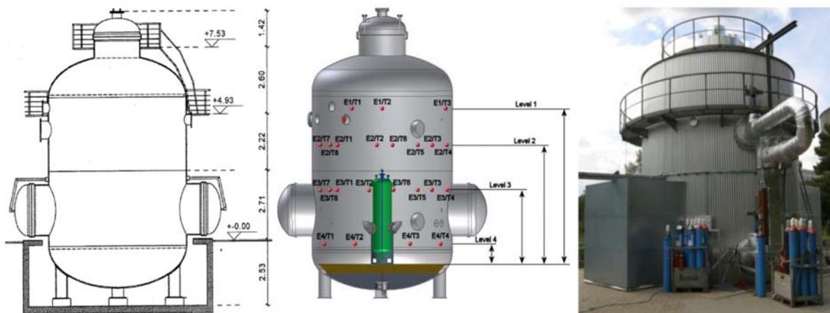
Figure 5. HYKA-A2 facility: main dimensions and side view
